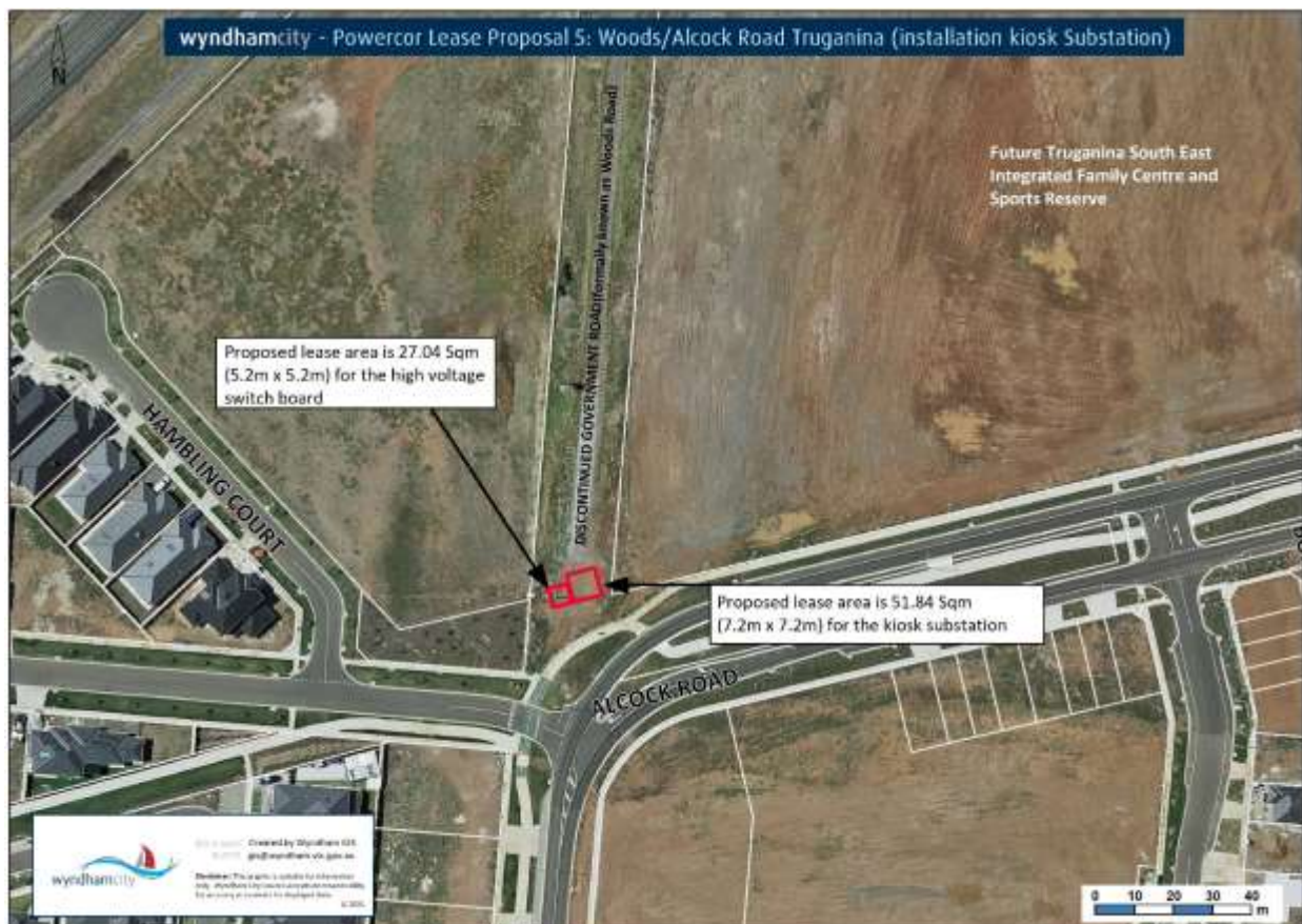
Figure 8. Aerial image showing proposed location of lease area for Kiosk Substation and Switch Board.
