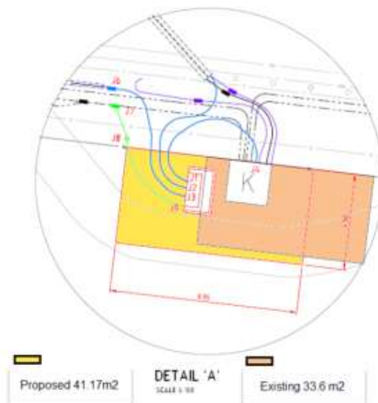
Figure 3. Plan showing proposed installation and upgrade of Switching Station at 9 Edgevale Way, Tarneit.
