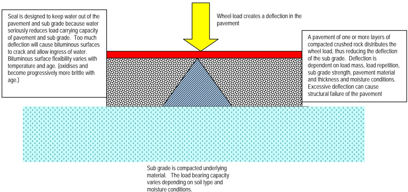
Pavement design is based on assessing these variables and adjusting the thickness and, if possible, quality of the pavement material to minimise the deflection. Traffic loads are based on both volume and weight, converting to equivalent standard axles (ESAs). Pavements therefore have an useful life defined by design, environmental, operating and maintenance conditions. A typical design life specified for lightly trafficked roads in council subdivision specifications is 20 years.
