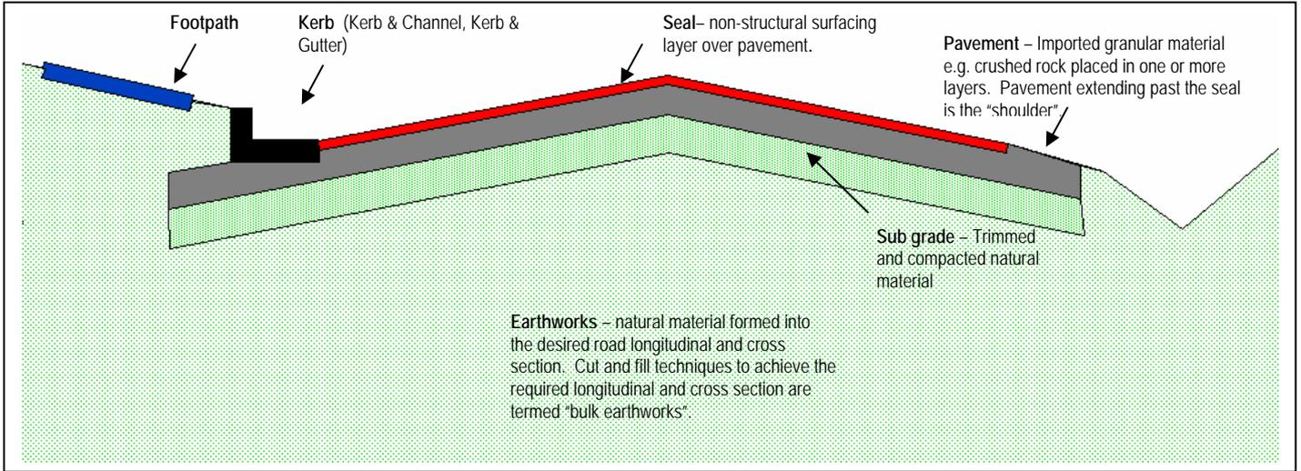
**Figure 12 Typical Gravel Road Cross Section Showing Components**
