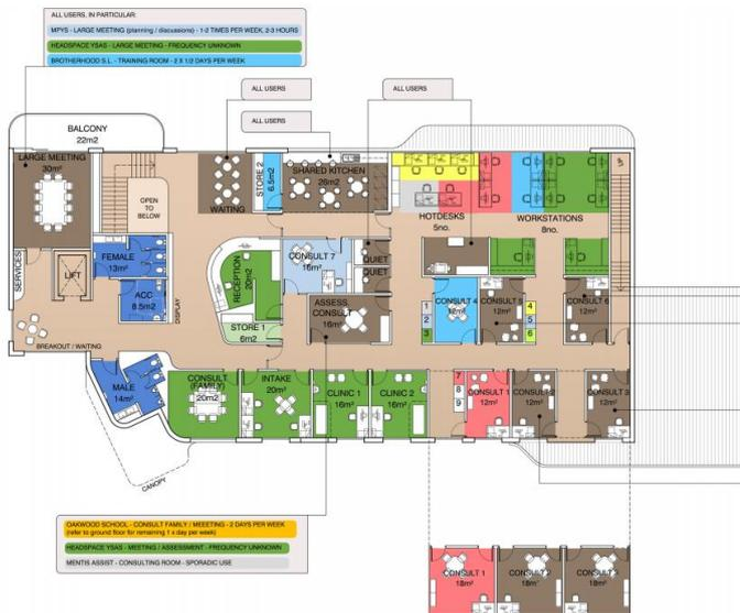
Figure 2: Concept design first floor
